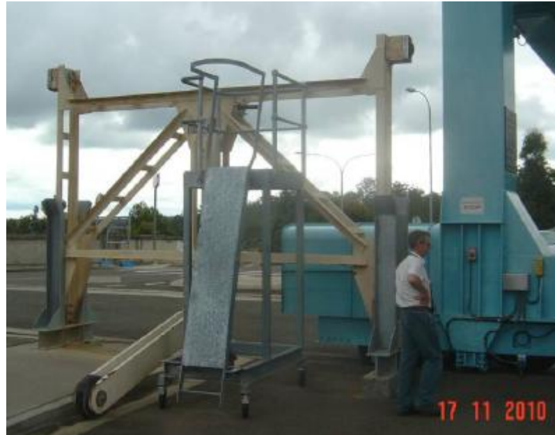
Figure 2: Lifting Frame for 2100mm Emergency Gate at Warragamba Dam
