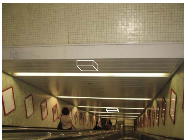
Figure 10 Indicative locations of CS154 loudspeakers in southern escalator tube
