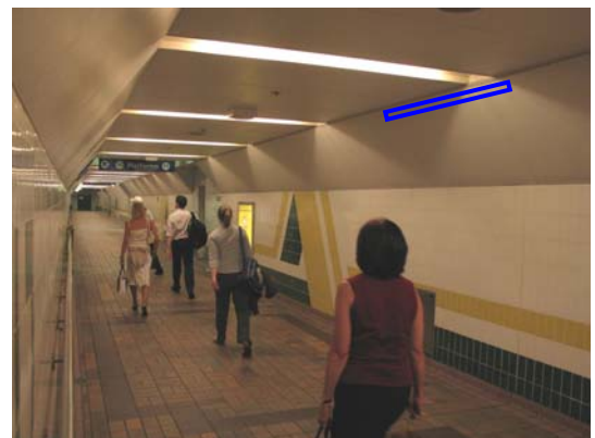
Figure 18 Indicative location of ALA07C loudspeakers in side wall of west section of Tunnel 3
